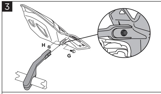
**Mount the cover (B) by the screw (G) and the nut (H).**
