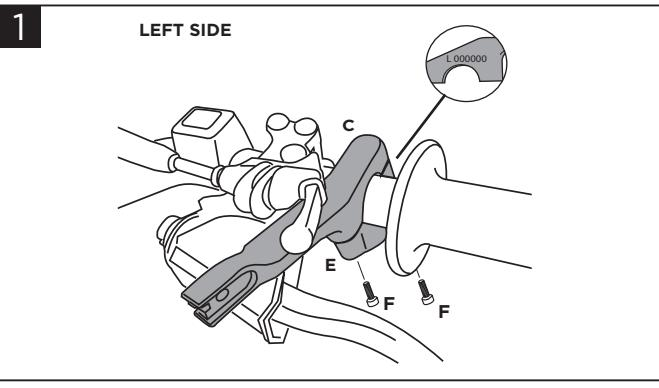
**Place the left-hand clamp (C+E), marked by the letter 'L', using the screws (F).**
