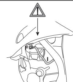
Mount the tank on the motorcycle and secure the hose (N) at the tap (F).
