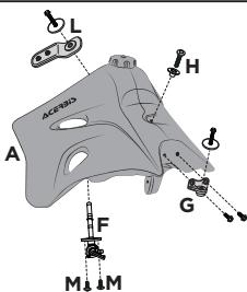
Remove the plastics and remove the original tank. Mount on the Acerbis tank (A) the original brackets (G) and (L) using the original screws and washers. Fit the original screw + bushing (H) on the tank. Finally, assemble the supplied tap (F) using the original screws (M).
