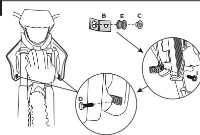
Insert the bushing (C) and the rubber (E) into the clips (B). Fix the clips (B) on the radiator using the screws (D) supplied and (I) original on both sides.
