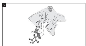
Reassemble bracket (M), bushings (Q), screws (P), grommet (L), bushing (I) and screw (O) on the Acerbis tank (A).
