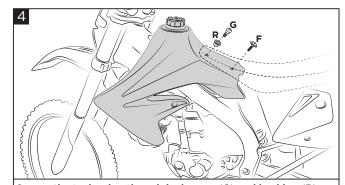
Secure the tank using the original screw (G) and bushing (R) and tighten the screw of the bike seat (F). Fissare il serbatoio tramite vite e boccola originali (G) ed (R) ed
