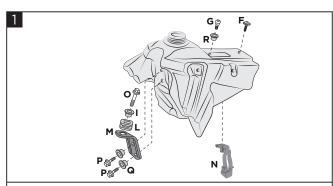
Remove the following parts from the original tank: bracket (M), bushings (Q), screws (P), grommet (L), bushing (I) and screw (O). Remove the screws (F), (G), the bushing (R) and the tap (N).
