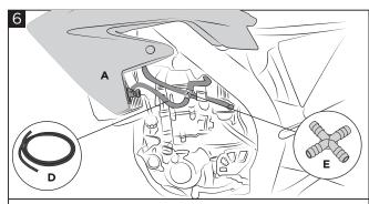
Cut the fuel hose to the right length, then attach it to the cross fitting (E) and the two provided taps (H), the original tap (N) and the carburetor.
