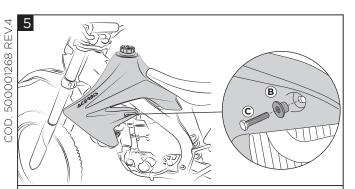
Attach the tank on both its sides using bushings (B) and screws (C).
