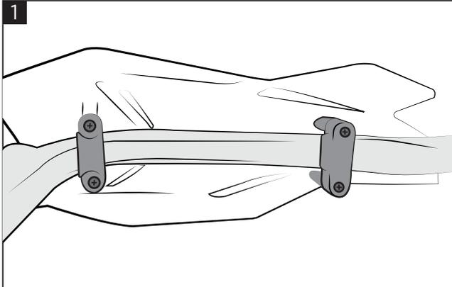
**Mount the bar on the cover with screws and brackets already supplied.**
