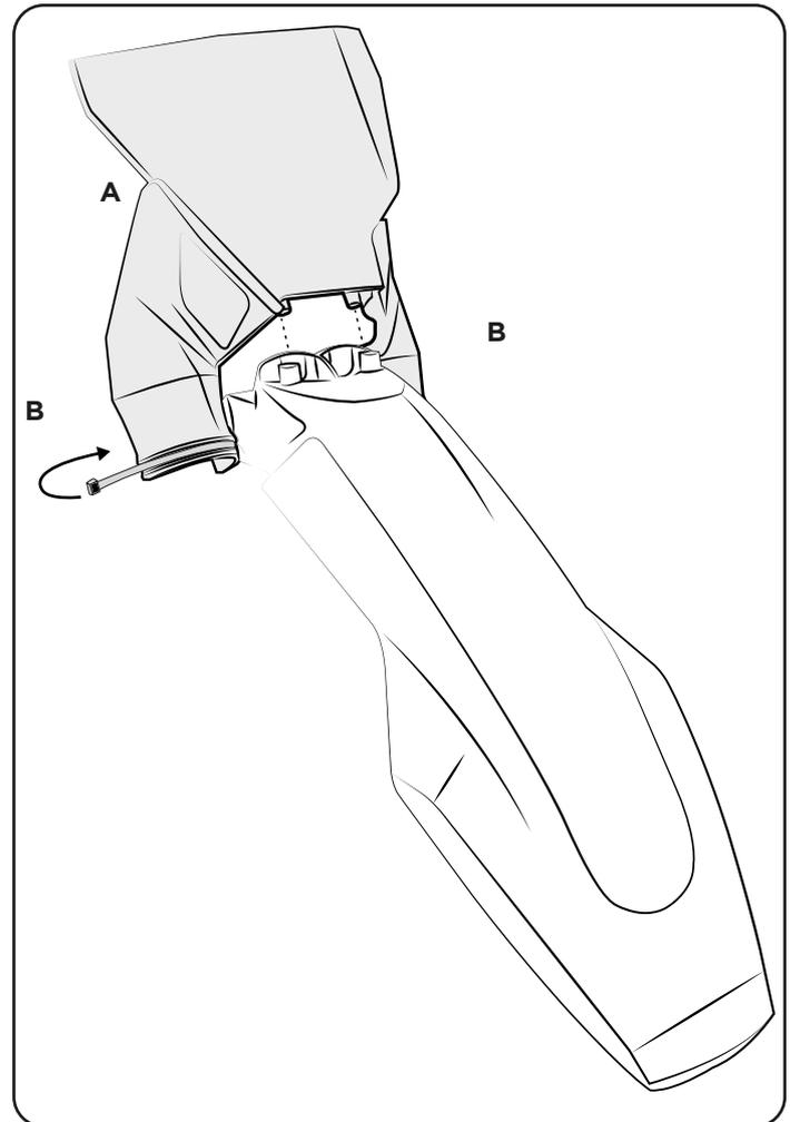
**1. Before assembling the front number plate, widen the 2 holes with a 9 drill bit to ensure the proper insertion.**
