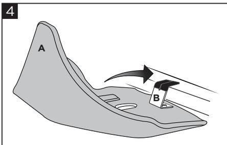
**Put the skid plate (A) being sure that the bracket (B) is inserted in the frame.**
