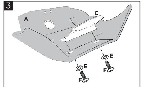
**Fix the bracket (C) to the skid plate (A) using the screws (F) and washers (E).**
