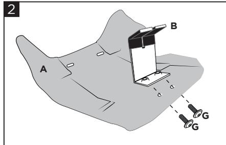
**Fix the bracket (B) to the skid plate (A) using the screws (G).**
