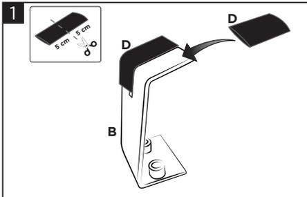
**Cut the rubber tube (D) (5 cm each side) and fit the bracket (B).**
