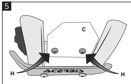
**Fix the bracket (C) to the frame using the screws (H).**
