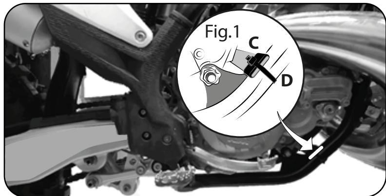
**1 - Cut the rubber tube (B) in half and add to the ends of the bracket (C) as indicated in the image. Do not cover the holes.**
