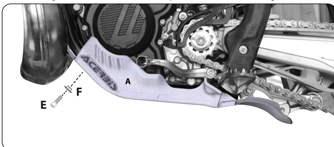
**6 - Secure the front of the skid plate with the bushing (F) and the screw (E)**
