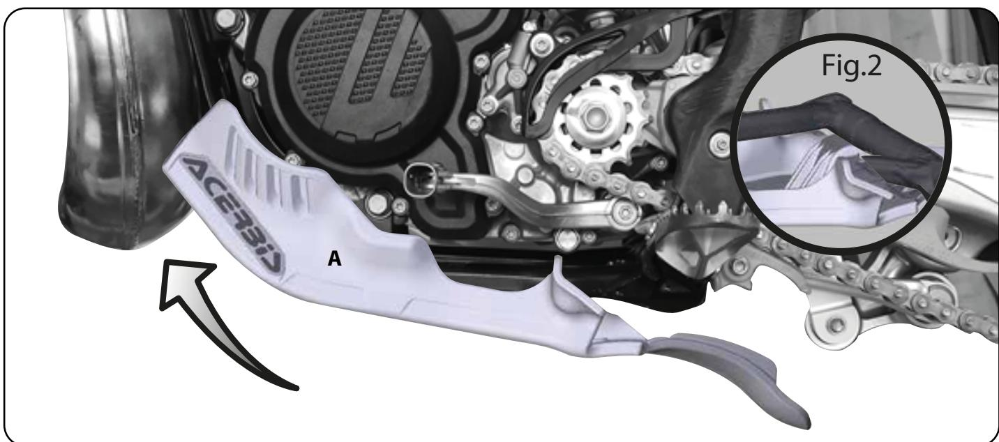
**3 - Place and push the skid plate (A) up and towards the front of the frame. ATTENTION! Make sure the hook on the back of the skid plate is not below the rear frame support tube. (figure 2 )**
