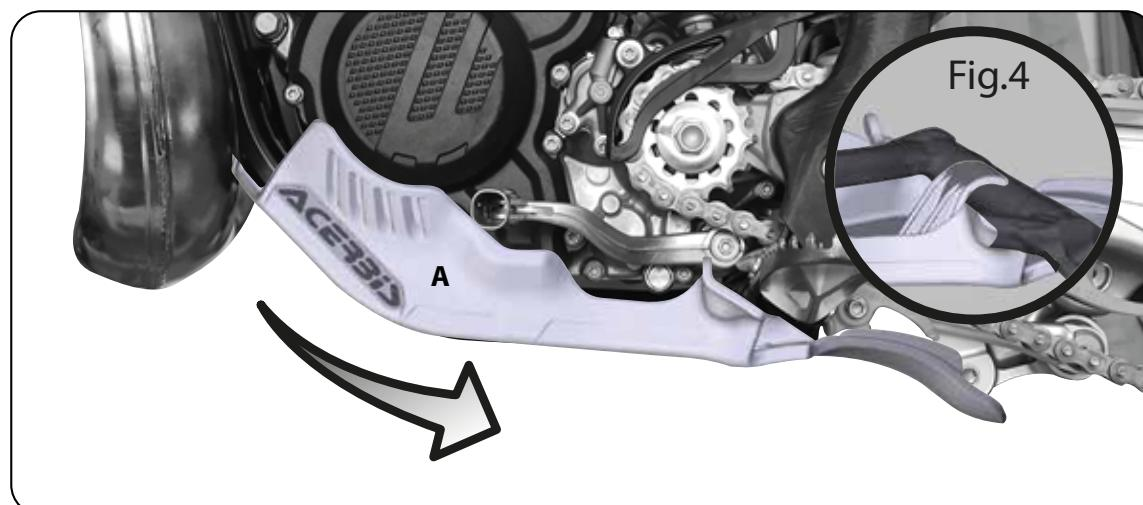
**5 - With force, push the skid plate (A) back towards the rear as indicated with the arrow. Make sure that the hook on the back of the skid plate is securely placed up and over the rear frame support tube. ( figure 4 )**
