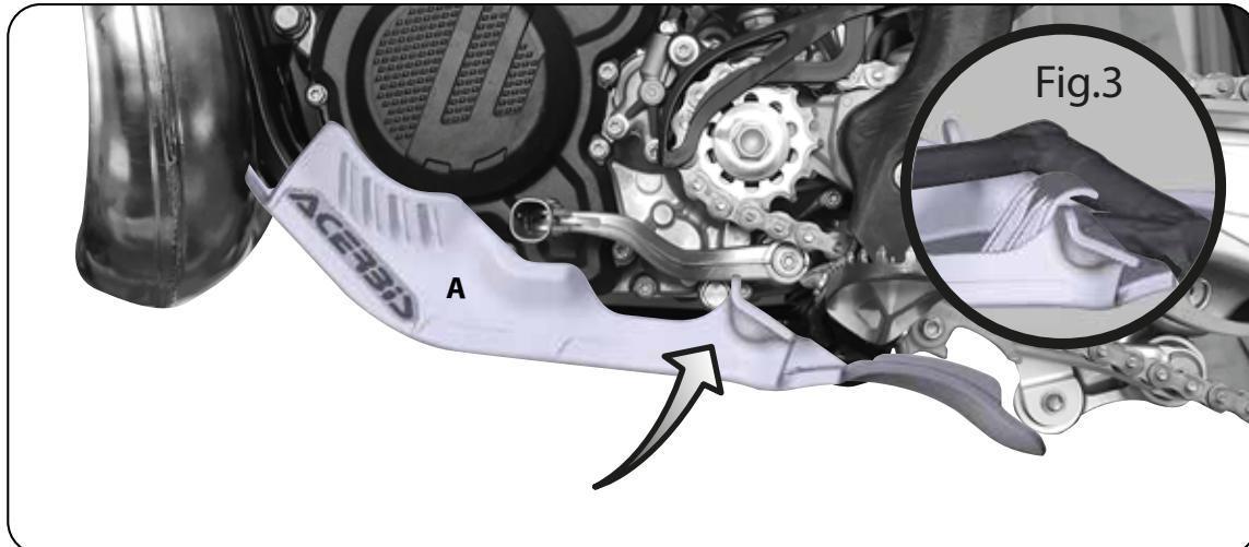
**4 - With force, push the skid plate (A) up towards the frame, where indicated with the arrow. Make sure that the hook on the back of the skid plate is above the rear frame support tube. ( figure 3 )**
