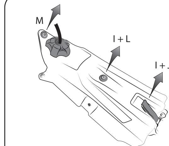
**2 - Disconnect the rubber clip (J), the (M) bolt, and the (I)+(L) bolt and bushing from the original tank.**
