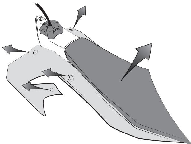
**1 - Remove the saddle and radiator shrouds from the stock tank.**
