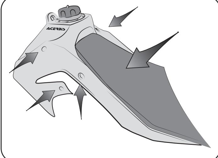
**6 - Install the radiator shrouds and then install the seat making sure all the bolts are tight.**
