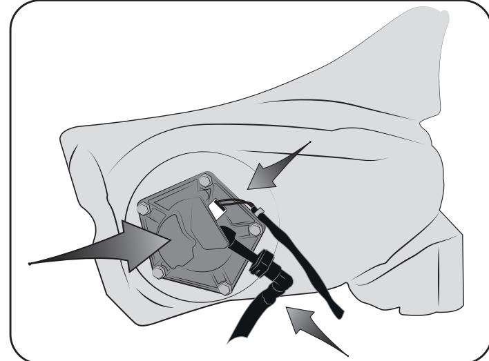
**4 - Mount the Fuel pump (F) into the Acerbis tank (A) and reconnect the wire harness and fuel line.**
