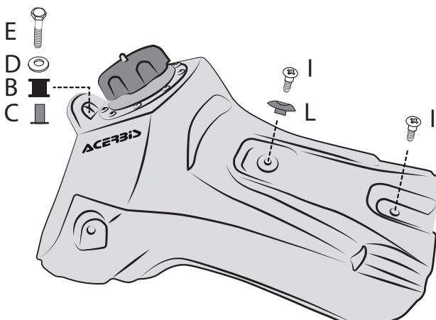
**5 - Insert the Rubber bushing (B) into the front mounting point on the tank. Then from the bottom insert the Metal bushing (C) into the bushing (B). Then from the top add the washer (D) and Bolt (E) and tighten the tank down onto the bike. Insert the seat screw and bushing (I)+(L) and re-connect the Rubber clip (J).**
