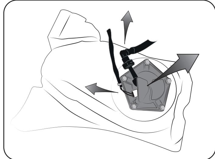
**3 - Raise the original tank and disconnect fuel line and wire harness from the fuel pump. Then empty any remaining fuel from the tank and remove the fuel pump (F) from the tank.**
