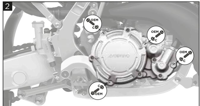
**Remove the four OEM clutch cover bolts as indicated in the image. Attach the X-Power cover (A) using the four OEM bolts and four bushings (C). Torque the bolts to the OEM suggested torque settings as indicated in your owner's manual. Then, re-connect the rear brake pedal by re-inserting the brake pedal bolt (E) and then torque to the OEM suggested torque settings as indicated in your owner's manual.**
