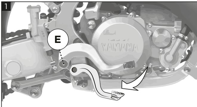
**To mount the X-Power clutch cover, begin by unscrewing the brake pedal bolt (E).**
