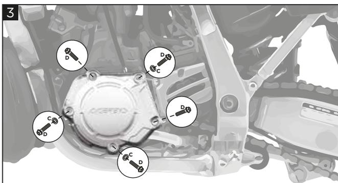
**Remove the five OEM bolts. Then install the X-Power ignition cover (B) using the four included bolts (D) and three bushings (C). Torque the bolts to the OEM suggested torque settings as indicated in your owner's manual.**
