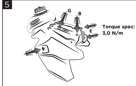
**Mount the Acerbis tank on the motorcycle. Tighten the screw (G) again. Retighten the screws (B+C) of the saddle and spoilers.**
