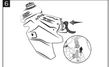
**Reconnect the fuel pump power cable and the fuel connector. Assemble the radiator scoops, side panels and seat.**
