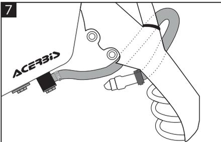
**Attach the HUSQVARNA fuel line to the Acerbis tank (A) as indicated in the diagram. Make sure the fuel line isn't folded over, obstructing the fuel flow.**
