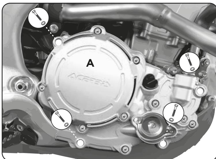
**Remove 4 OEM clutch cover bolts exactly as indicated in the image above. Attach the X-Power clutch cover utilizing the 4 OEM bolts and 4 of the included (C) bushings and then tighten to the manufacturers suggested torque settings as indicated in the owners manual. Re-install the rear brake bolts and tighten them to the manufacturers suggested torque settings.**
