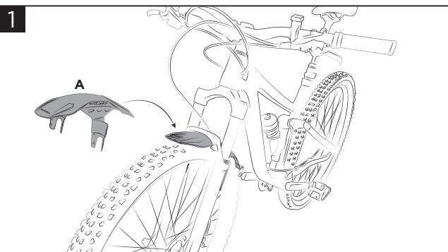
**Place the front fender (A) on the bike in order to decide where to drill it (by choosing among the drilling positions shown on the front fender).**
