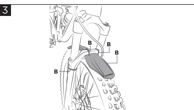
**Place the front fender after drilling the holes. Then, fix it using the provided cable ties (B).**
