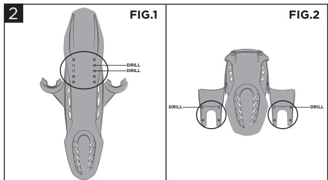
**Drill either the holes among those shown in figure 1, as decided before. Repeat the drilling operation on the forks sides.**
