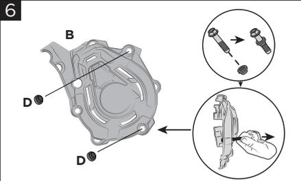
**6** Before assembling the X-Power (B), block the bushings (D) inside the protection. In order to ease the mounting, it is recommended to use a screw by inserting it in the bushings. Then pull the screw until the bushings are stuck in their plastic seat. Finally, remove the screw.
