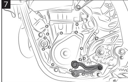
**7** Lower the gear shift by putting the bike into the first gear. Place the protection (B) on the engine casing.
