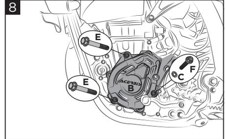
**8** Mount the X-Power clutch protection (B) with the washers (G), the screws (E), the original screw (F) and the bushing (C). Closing torque as reported on the original instructions manual of the bike.
