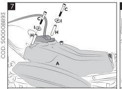
Secure the fuel tank (A) using the bushings (H), the washers (I) and the screws (C). Fissare il serbatoio (A) tramite le boccole (H), le rondelle (I) e le viti (C).
