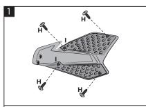
Mount the spoiler (I) through the screws (H). Montare gli spoiler (I) tramite le viti (H).
