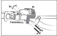
OLNY FOR TWINWALL HANDLEBAR Position the bracket (B<sub>1</sub>) in the indicated position and fix it by closing with the collar (B2) through the screws (F).
