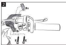
Position the bracket (B<sub>1</sub>) in the indicated position and fix it by closing with the collar (B<sub>2</sub>) through the screws (E).
