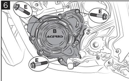
**Mount the X-Power ignition protection (B) with the screws (E). Closing torque as reported on the original instructions manual of the bike.**
