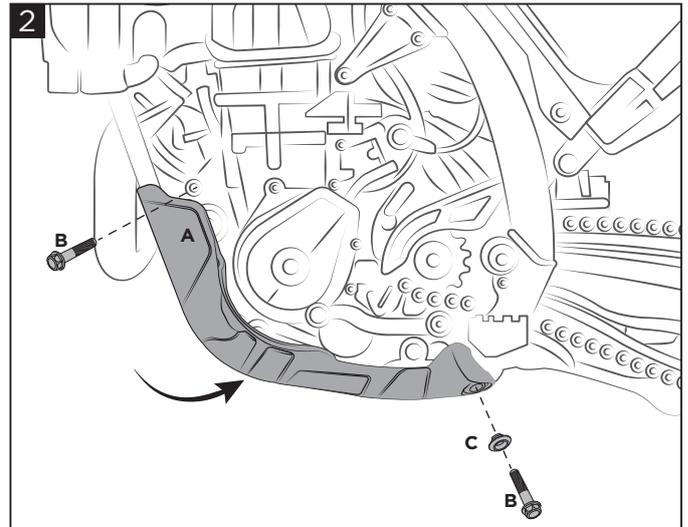
**Position the Acerbis skid plate (A) and fix it using the supplied screws (B) and the bushings (C).**
