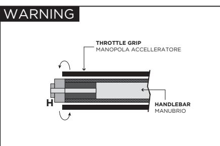
**After fixing the screw (G) make sure the throttle grip do not create friction with the spacer (H).**
