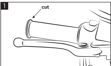
**Cut the end of the grip so that it can access the internal insert.**
