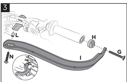
**Fix the bar (I) to the handlebar using the spacer (H) and screw (G) as shown in the figure. Fix the bar to the bracelet using the screw (N) and the bushing (L).**
