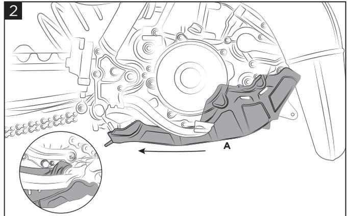
**With force, push the skid plate (A) back towards the rear as indicated with the arrow.**
