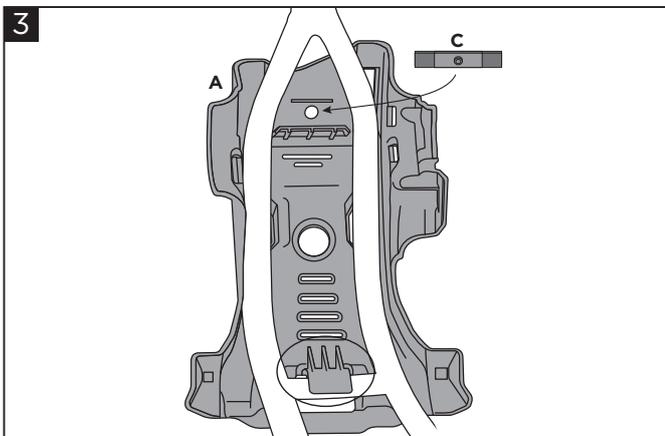
**Make sure that all the hooks of the skidplate are well engaged at the frame and lay the bracket (C) into the appropriate seat.**
