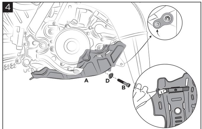
**Secure the skid plate (A) to the frame using the screw (B) and the bushing (D) holding the bracket still with your finger, using the hole in the skid plate, as shown in the figure. Then re-insert the silent block.**
