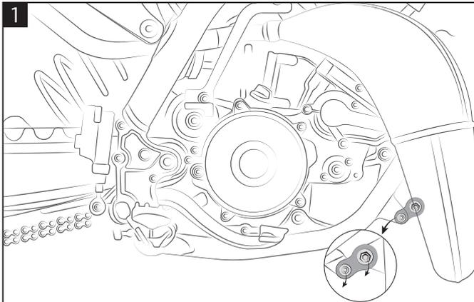
**Remove the silent block through the 2 screws.**
