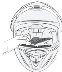
Pull by releasing the nose guard.
