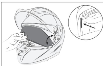
To remove the visor, pull it outwards. To reassemble it, carefully hook it into the special supports.
