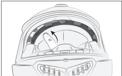
Hook the cap by inserting the plastic part in the appropriate spaces along the frame.
