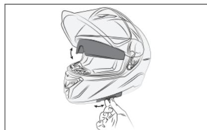
Raise and lower the visor, as shown in the figure, using the appropriate slider.
