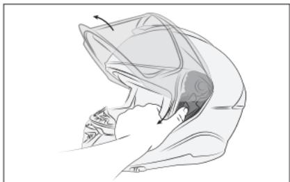
Remove the visor by unhooking it using the special support.
