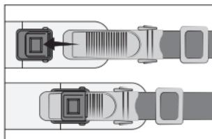
**A** - Once you are wearing the right size Acerbis helmet (closely following the instructions above) firmly tighten the chinstrap by passing the end of the ribbon through the "D" shaped rings. Now pass the end of the ribbon over one of the "D" rings and through the second one (as shown in fig. A) then pull it until it is comfortably stretched. To release the chinstrap, pull the red ribbon attached to one of the "D" rings and remove the ribbon as shown in fig. A.
