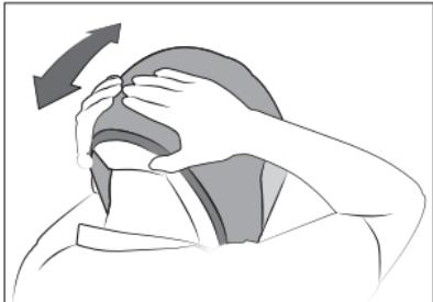
Fasten the helmet and with one hand hold the chin strap and with the other hand try to remove the helmet with force from the back. If the helmet can be easily removed, the size is wrong or it is not worn and fastened properly.
