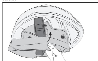
Insert the pillow into the strap and then re-attach the buttons and the velcro.
