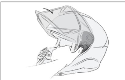
Attach the visor using the special support.
