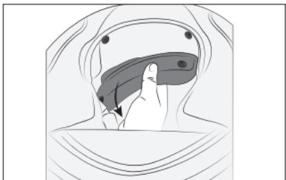
Remove the cap by unhooking the back part from the buttons and take it off.
